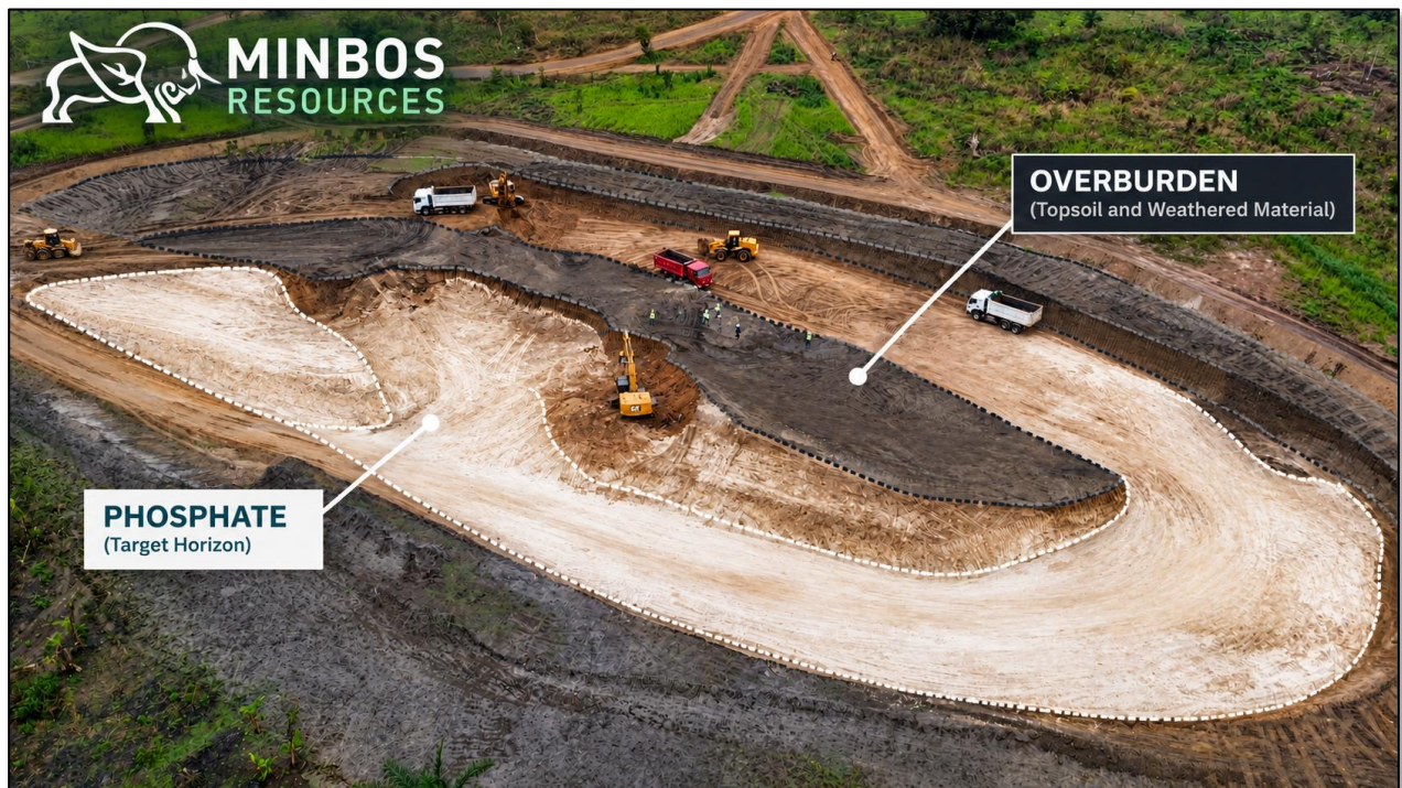
Figure 1: Aerial view of open-cut bench development and haul-road alignment at the Cacata Phosphate Deposit.
