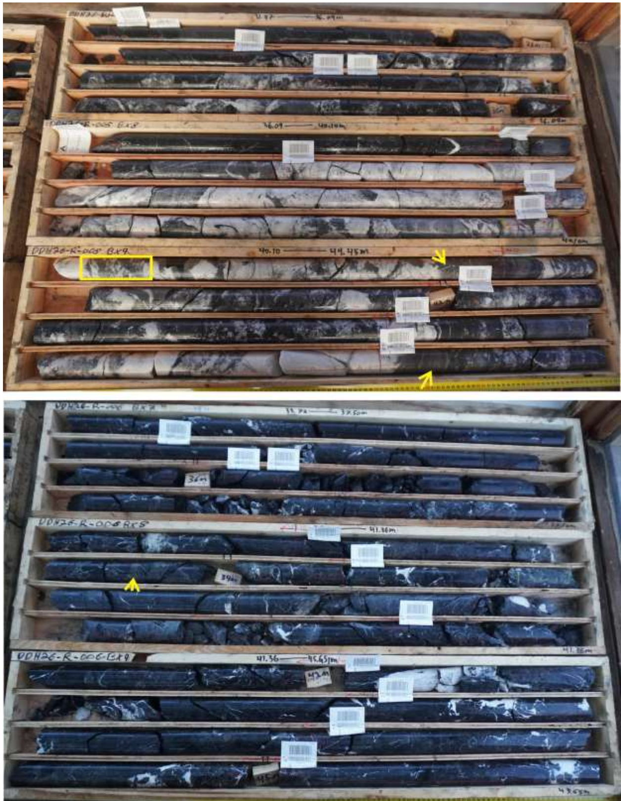
Figure 3: Core trays (wet) from DDH26-PR-005 (31.97–44.45m, top) and DDH26-PR-006 (33.72–45.65m, bottom), Pad 2, showing white barite–quartz with sphalerite–galena. Yellow arrows indicate clusters of high sphalerite abundance; the yellow box marks the core shown in Figure 4, right. Mineralised intervals are visual observations only; assays pending.
