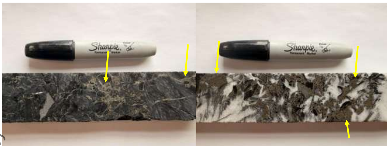
Figure 4: Cut drill core from Pad 2, annotated by HEG: (left) DDH26-PR-006, 49.7m, honey-brown sphalerite as breccia cement and infill in black fossiliferous Dunedin Formation limestone, flanking the upper contact of the quartz-barite zone; (right) DDH26-PR-005, 40.1m, honey-brown sphalerite \pm galena in white quartz-barite cement at the Dunedin/Stone Formation contact. Arrows indicate sphalerite; visual observations only; assays pending.
