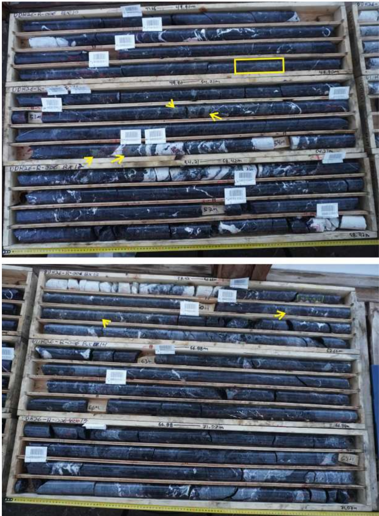
Figure 3 (continued): Core trays (wet) from DDH26-PR-006 (45.65–58.42m, top; 58.42–71.07m, bottom), Pad 2. Yellow arrows indicate clusters of high sphalerite abundance; the yellow box marks the core shown in Figure 4 , left. Mineralised intervals are visual observations only; assays pending.
