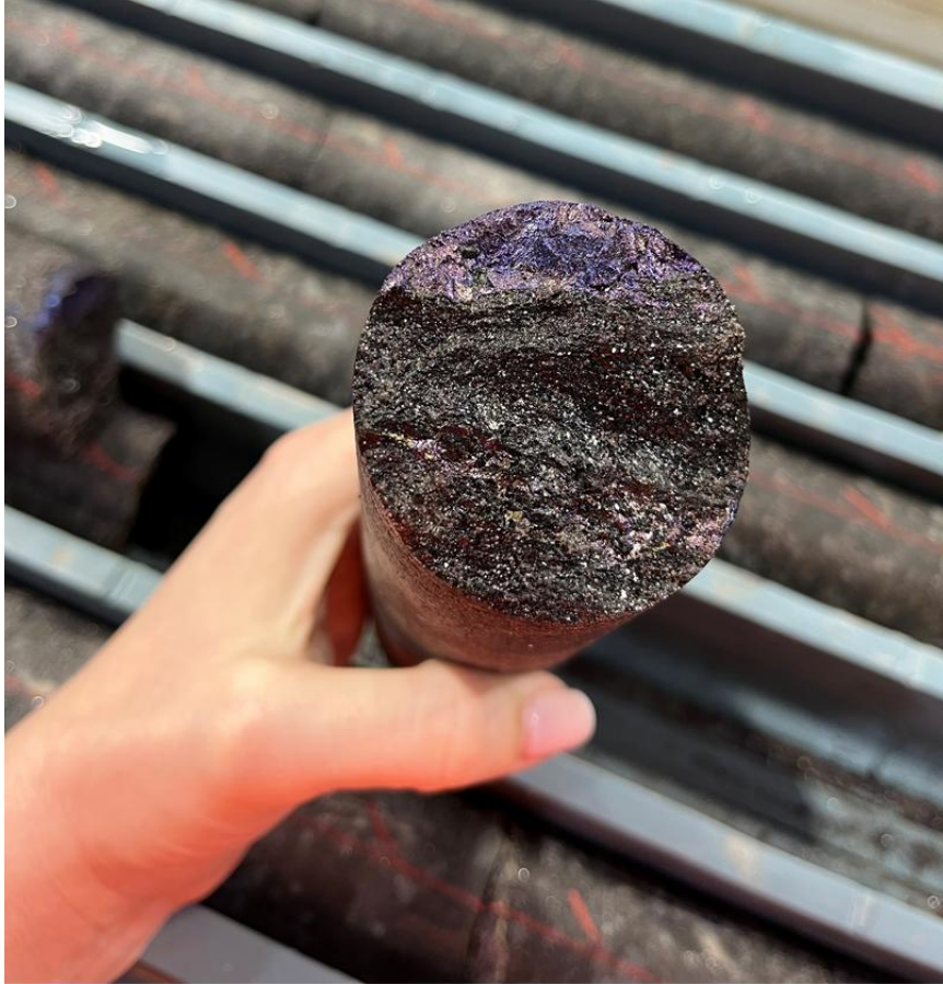
Figure 3: Bornite Mineralisation (purple) observed in 26KVUG0944 at 292.50m Downhole
