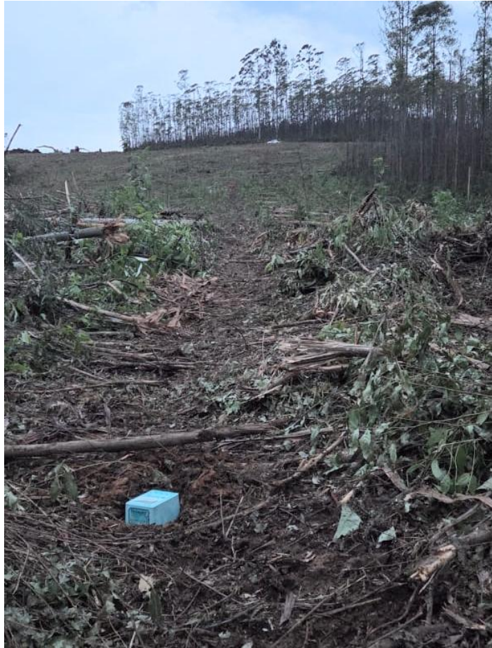
Figure 3. Tromino passive seismic unit on site near Morro do Ferro. The plantation trees have only recently been logged. The unit is slightly buried to reduce noise affects of wind. The units take measurmnts from 30 to 40 minutes for each station.
