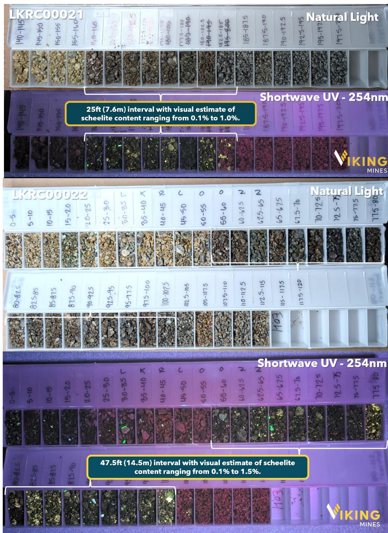
Figure 1; Chip trays from LKRC00021 & LKRC00022 photographed under shortwave UV light (254nm) and natural light. Sample intervals are labelled in feet downhole. Visible scheelite (fluorescing) was logged from 160ft to 185ft (48.8m to 56.4m). Assay results expected in approximately 6-8 weeks.
