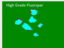
Laser ore-sorting technology by TOMRA applied to Quinn Project metallurgical samples, showing clear differentiation of ore types and waste. Samples approximately 10-15mm
