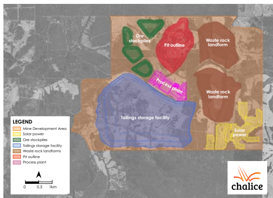
Figure 4. Gonneville MDA preliminary site layout.
