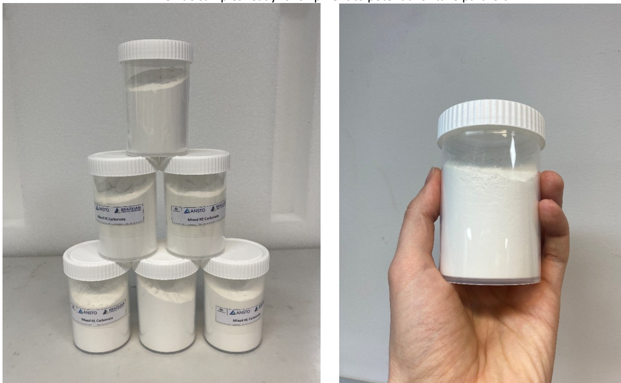
Figure 9: ANSTO produced MREC product containing on average approximately 52% by volume TREO 15 . Oxide samples ready for shipment to potential offtake partners.
