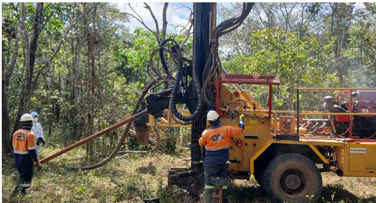
Figure 4: AC drilling at West Mwombezhi
