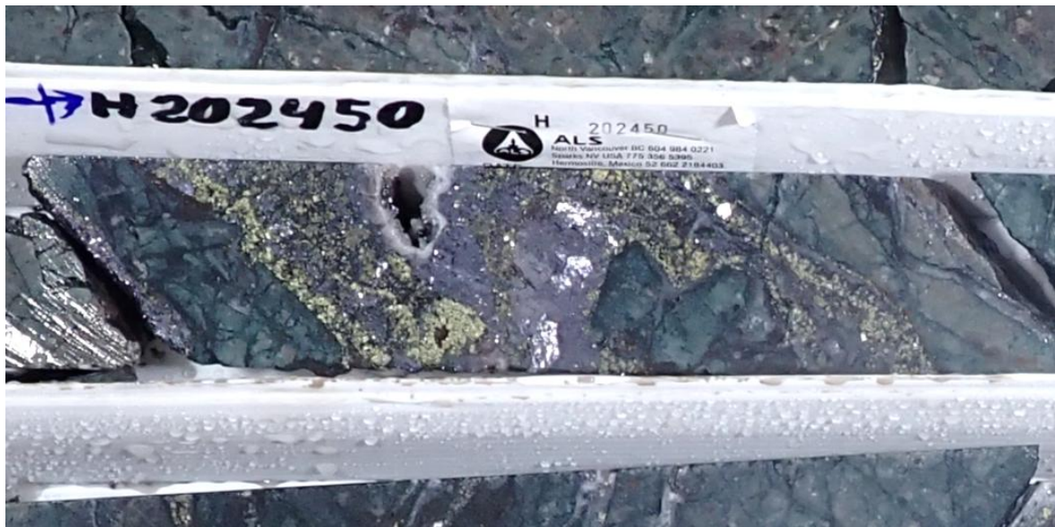
Figure 2. Cut core from GV-26-008 from ~102.7 to 103.0m down hole, showing semi-massive coarse grained galena (grey), with lesser low-iron sphalerite (pale yellow) and minor chalcopyrite (bright yellow) and quartz (white) in a chloritic andesite breccia. This interval returned 1.2m at 45g/t Ag, 3.4% Zn, 5.7% Pb & 0.3% Cu from 102.7m.
