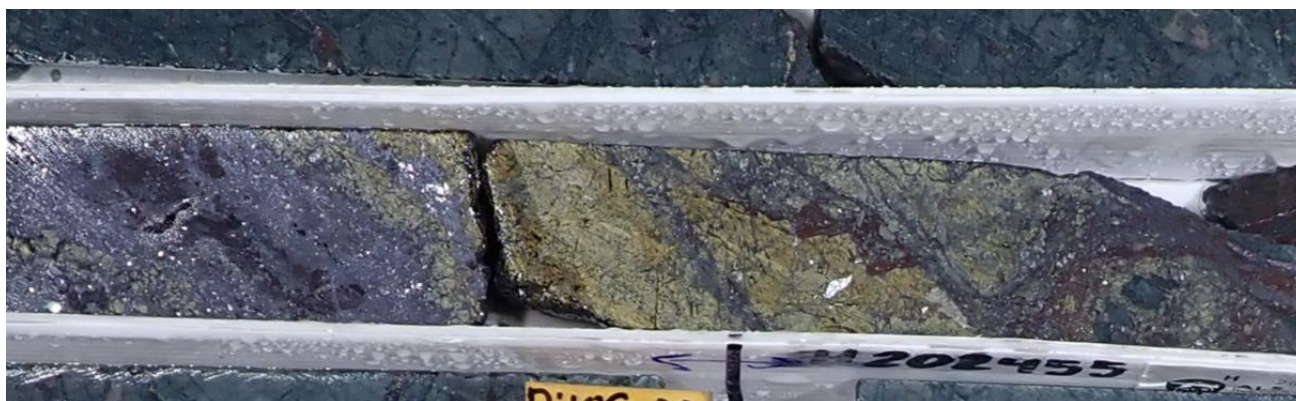
Figure 4. Cut core from GV-26-008 from ~107.3 to 104.7m down hole, showing massive galena (grey), low-iron sphalerite (pale yellow) and hematite (red-brown) mineralisation. This interval returned 1.0m at 76g/t Ag, 17.0% Zn & 14.6% Pb from 107m.
