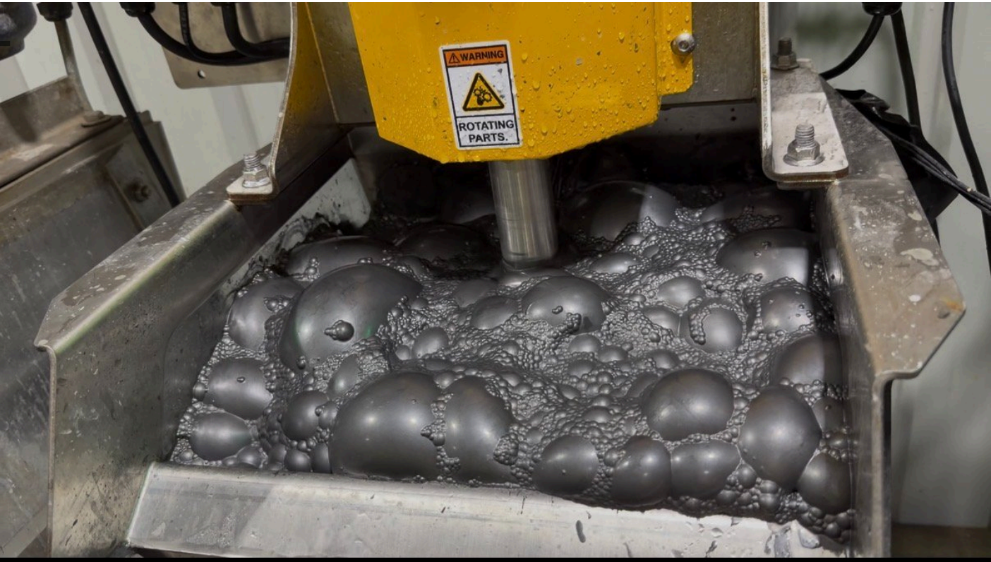
FIGURE 4 — SULPHIDE FLOTATION, REMOVAL OF GANGUE SULPHIDE MATERIAL
