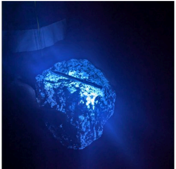
FIGURE 8 — ROCK CHIP FROM THE BULK SAMPLE ZONE, 16.9 KG GRADING 64.3% WO 3 , UNDER UV LIGHT
