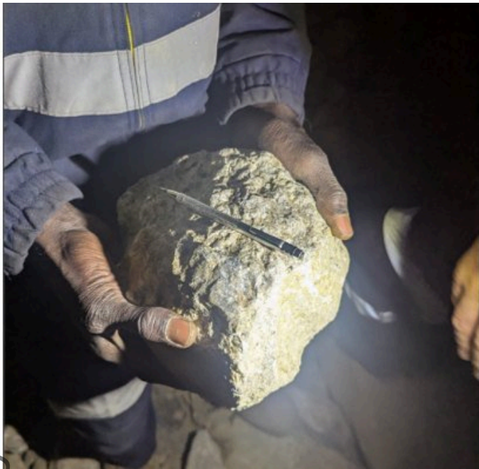
FIGURE 8 — ROCK CHIP FROM THE BULK SAMPLE ZONE, 16.9 KG GRADING 64.3% WO 3 , UNDER UV LIGHT
