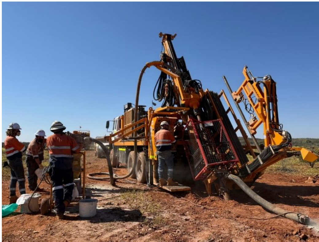
Figure 1 RC drill rig at Errabiddy Gold Project
