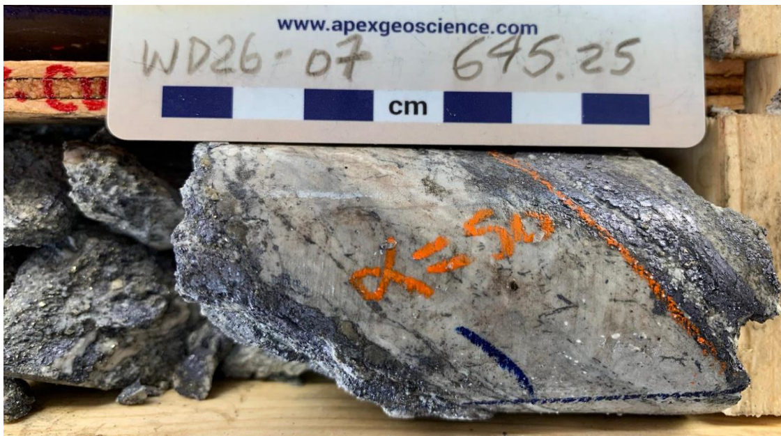
Figure 5: Very strongly mineralised visual molybdenite (blueish-grey)-quartz-pyrite veining in NQ drill core from approximately 645.25m downhole in drill hole WD26-07. Laboratory assays for this interval are pending.
