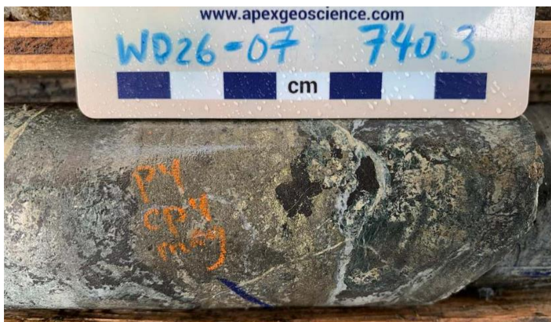
Figure 3: Very strong visual chalcopyrite (brassy)-pyrite (yellowish)-magnetite (black) in NQ drill core from approximately 740.3m downhole in drill hole WD26-07. Laboratory assays for this interval are pending.
