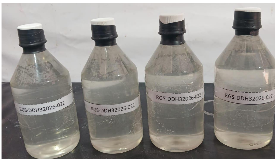
Figure 3 – DDH-3 Brine Sample Number 20 Collected from Packer Testing
