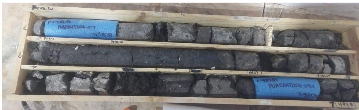
Figure 2 – DDH-3 Core Showing Brine-Bearing Lithology at Depth
