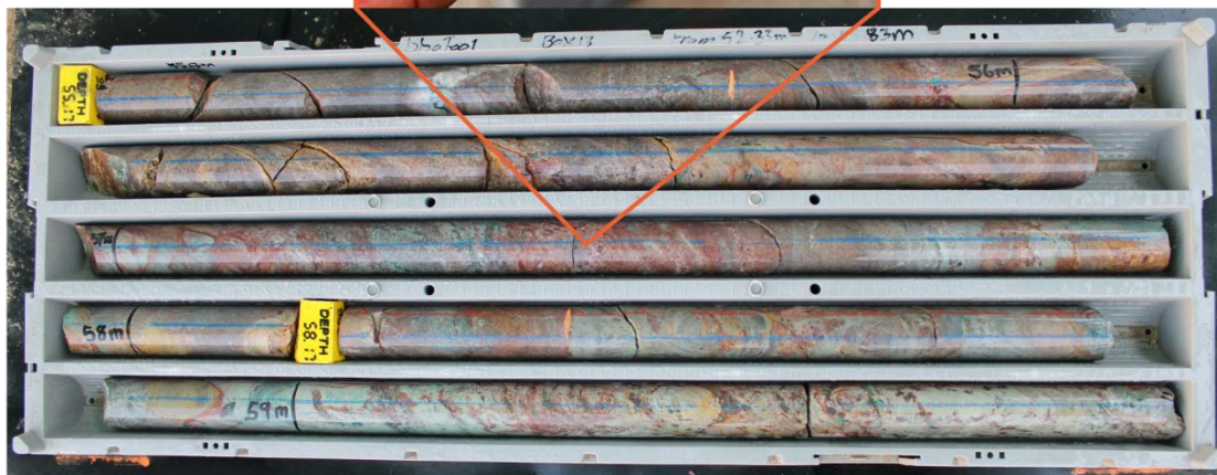
Figure 5 - DDOT001 Core from 52.33m to 59.83m, showing a selection of mineralised drill core from ~57.58m, with the visually identified copper minerals annotated. Refer to Appendix A for details.
