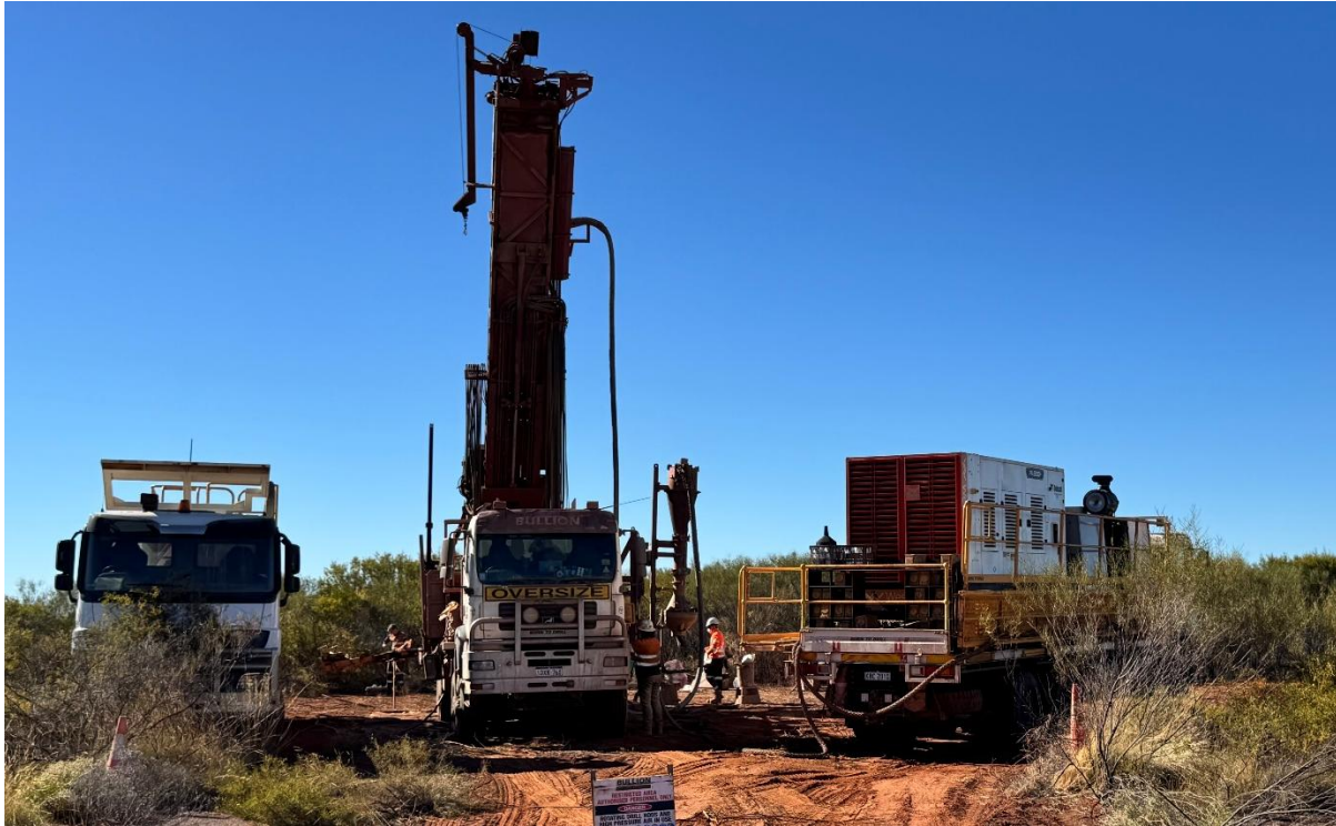
Figure 3 – Resource definition drilling at the Jims Gold Deposit
