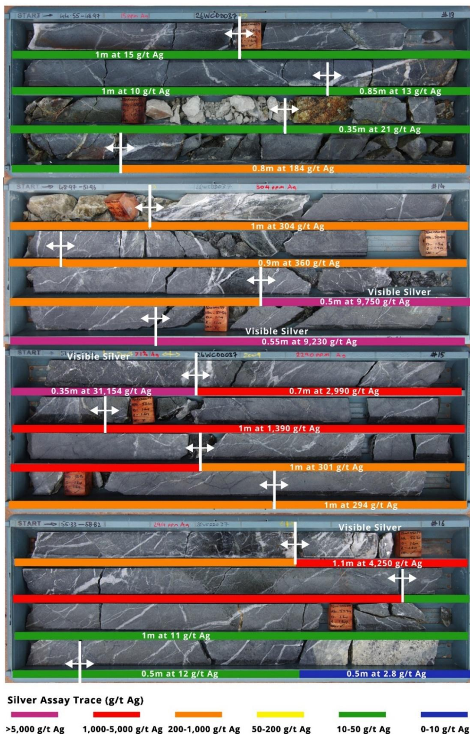
Figure 3. Diamond drill cut core photograph of 26WCDD037 from 44.55m to 58.82m downhole depth highlighting visible native silver hosted in fracture fill quartz-carbonate veining within ultramafic, and corresponding assay results (See Appendix 3).
