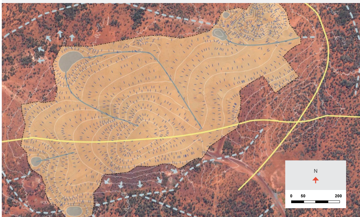
Geomorphic design of Monty waste rock deposit
