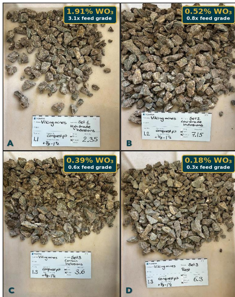
Figure 2; TOMRA XRT sorted fractions from the Conquest Pit sample with assayed grades: A: Set 1 High Grade Inclusions (1.91% WO 3 ), B: Set 2 Low Grade Inclusions (0.52% WO 3 ), C: Set 3 CONTAIN™ Inclusions (0.39% WO 3 ) and D: Low-grade (0.18% WO 3 ) (clockwise from top left).
