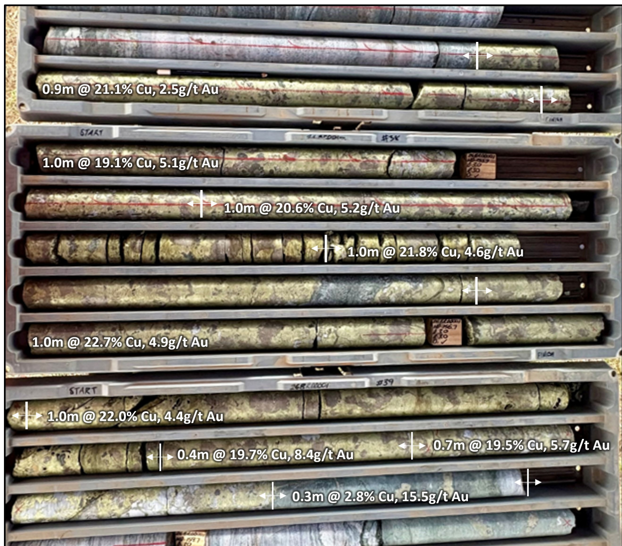
Figure 2. Drill core photos of the massive chalcopyrite interval in BRDD001 (individual samples illustrated on image taken from 152.1m to 159.4m – full details in Appendix 1, Table 1).
