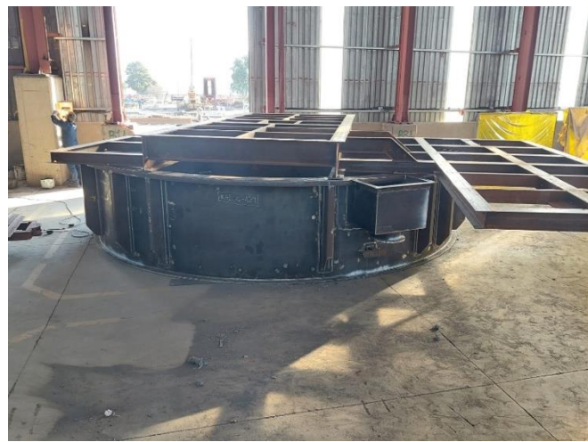
Figure 9: CIL Tank fabrication
