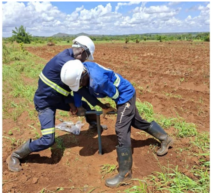
Figures 2 & 3: NGX's Malawi team hand augering and logging at its Msinja Licence.
