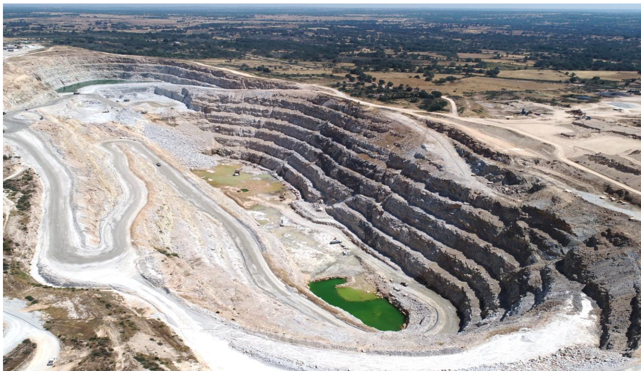
Northern area of the pit and temporary sump. Operations are currently mining Phase 6 at elevation 645 RL, with ore grade increasing. 8 July 2026.
