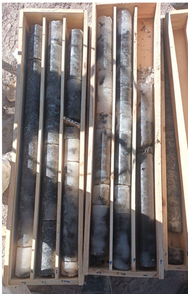
Figure 3 – Representative drill core from DDH-3 showing halite-rich horizons and basin sediments interpreted to host lithium-bearing brines.
