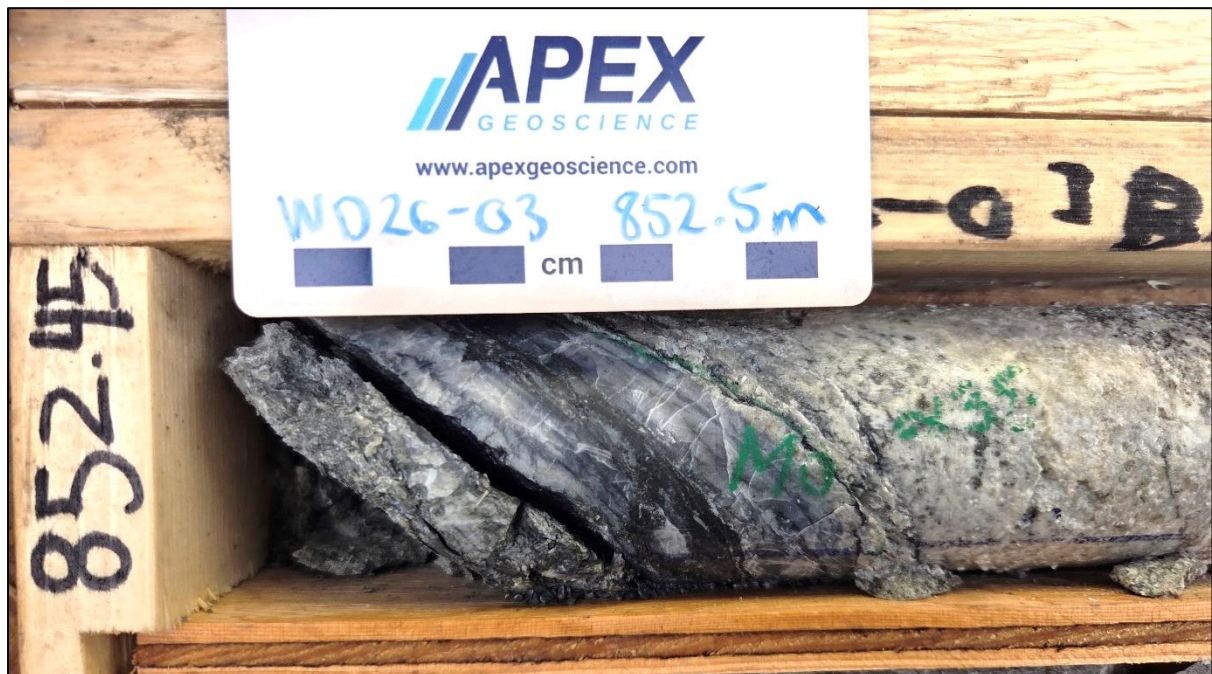
Figure 1: Very strong visual molybdenite (blueish-grey)-quartz-pyrite veining in NQ drill core from approximately 852.45m downhole in drill hole WD26-03. Laboratory assays for this interval are pending.
