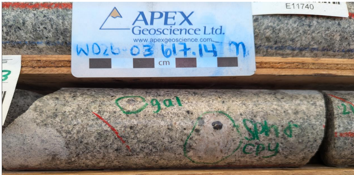
Figure 3: Weakly altered endo-skarn with visual sphalerite, chalcopyrite, and galena in NQ drill core from approximately 617.14m downhole in drill hole WD26-03. Laboratory assays for this interval are pending.
