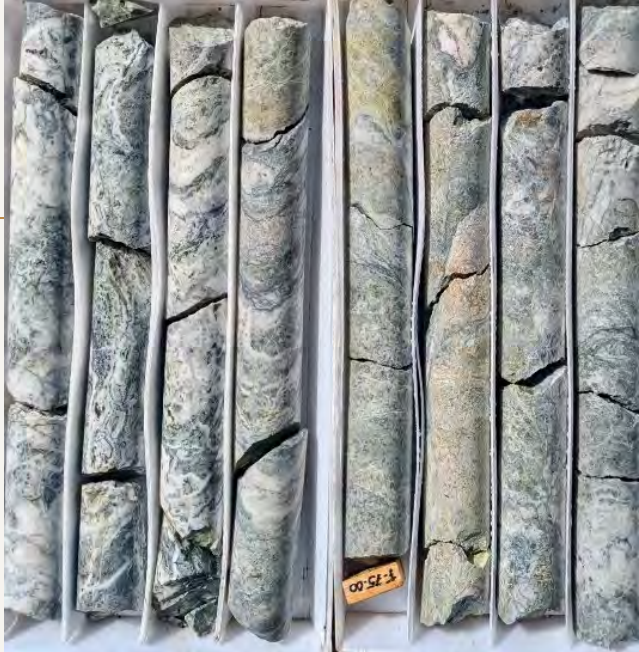
1 Banded quartz vein in dill core. CDH-152: 1.98m @ 4.59 g/t gold, 520 g/t silver from 18.5m (left) and CDH-154: 1.90m @ 1.83 g/t gold, 305 g/t silver from 75.1m (right).
