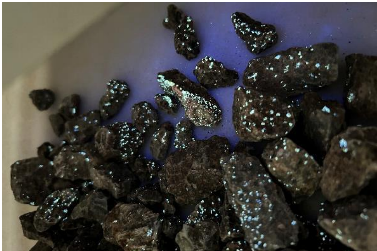
Figure 1; High-grade sorted fraction (Set 1) from the Conquest Pit sample under ultraviolet light, showing characteristic blue-white fluorescence of scheelite. Visual estimate containing between ~1.5% to ~3.5% scheelite (~1.2% to ~2.8% WO 3 ). Refer to Appendix 1. Assay results expected late July 2026.
