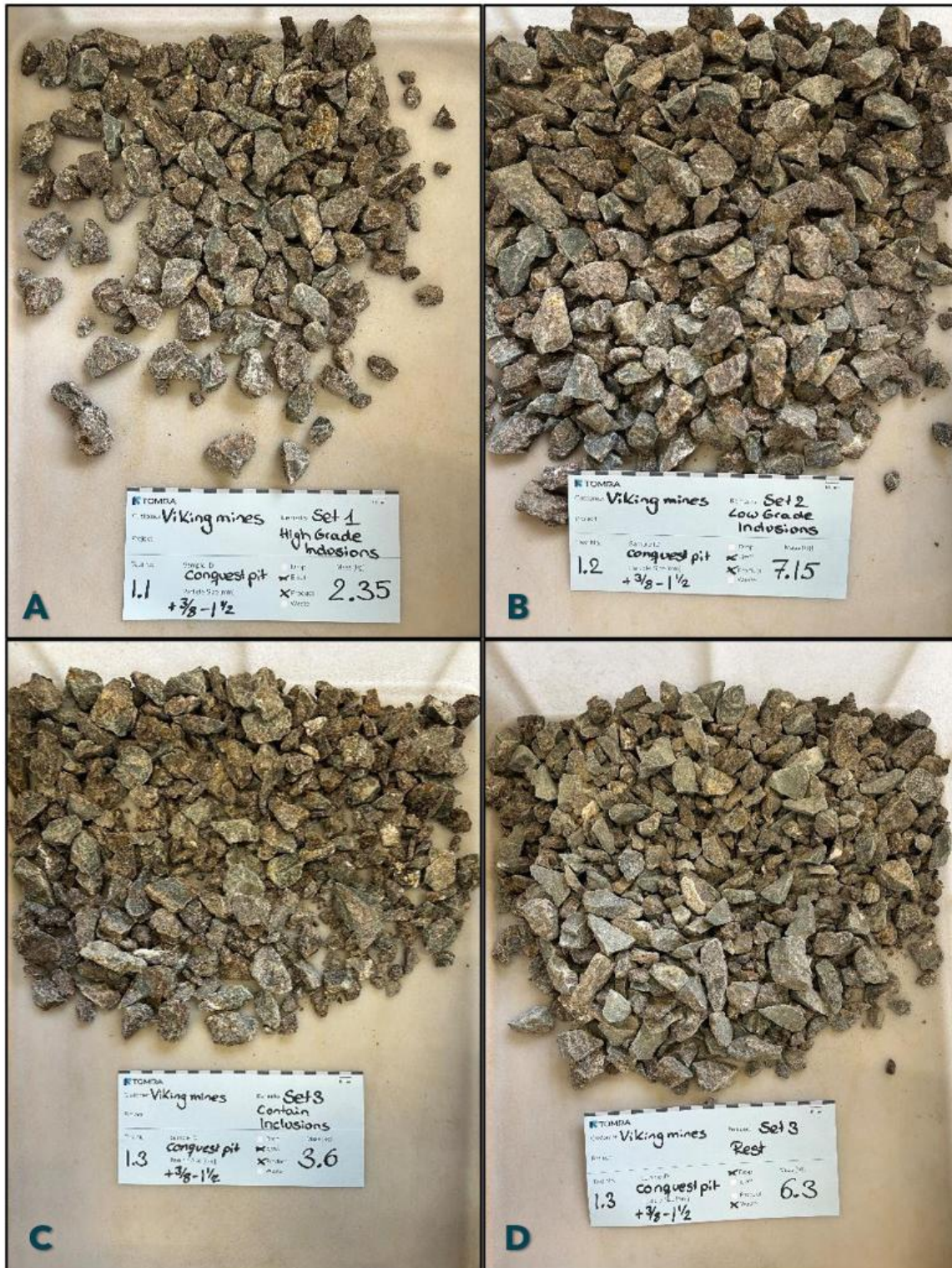
Figure 2; TOMRA XRT sorted fractions from the Conquest Pit sample: A: Set 1 High Grade Inclusions, B: Set 2 Low Grade Inclusions, C: Set 3 CONTAIN™ Inclusions and D: Waste (clockwise from top left).
