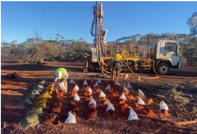
Photo 1: Star West alluvial workings and Penny's Fault aircore samples.
