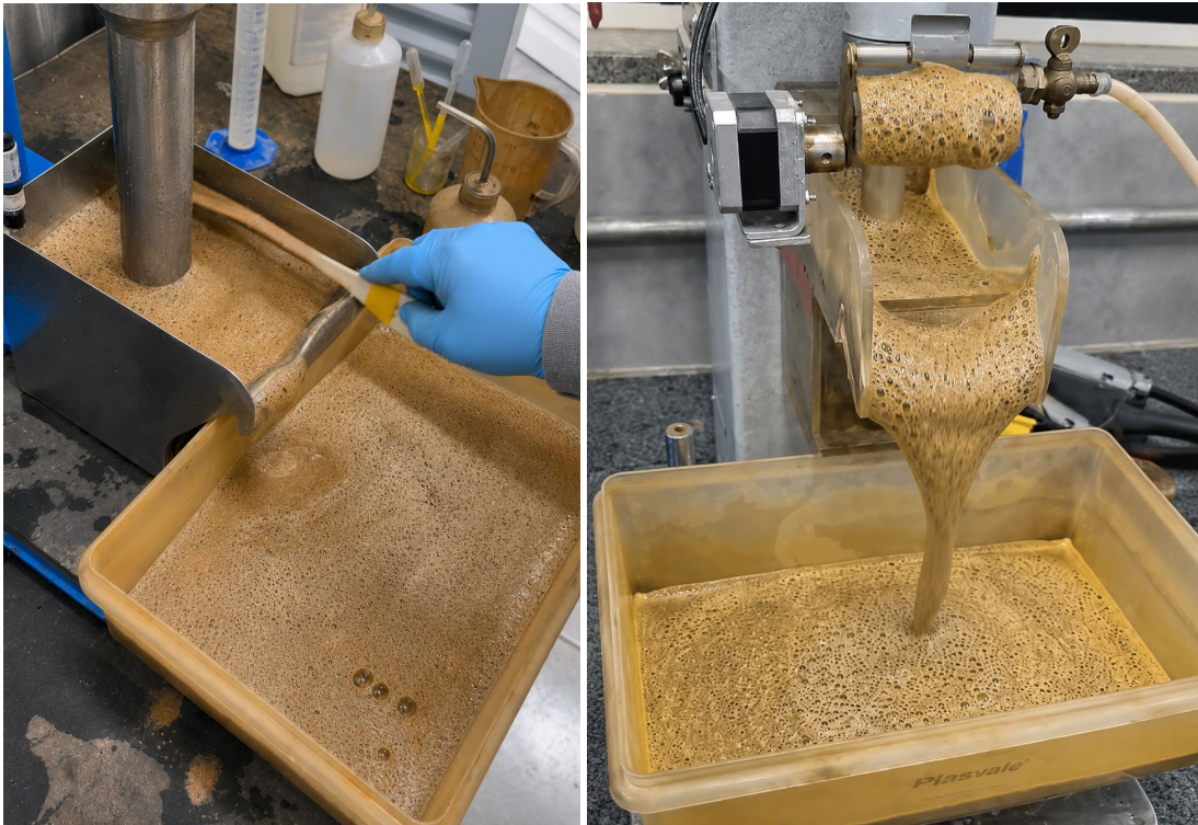
Figure 2 – niobium flotation by CIT-SENAI. On left: niobium flotation (second cleaner stage). On right: niobium flotation (third and last cleaner stage – the more yellow colour reflects cleaner material).
