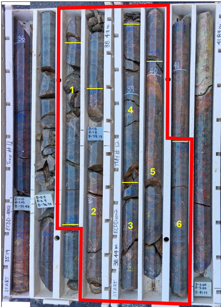
Figure 6: Mountain Pass-type LREE-enriched mixed carbonatite intersected in drill hole ECDD0002 with intercept (outlined in red) of 3.75m grading 4.45% TREO from 37.00m to 40.75m, including 0.7m grading 6.03% TREO from 40.05m to 40.75m (see Appendix III for assay results).
