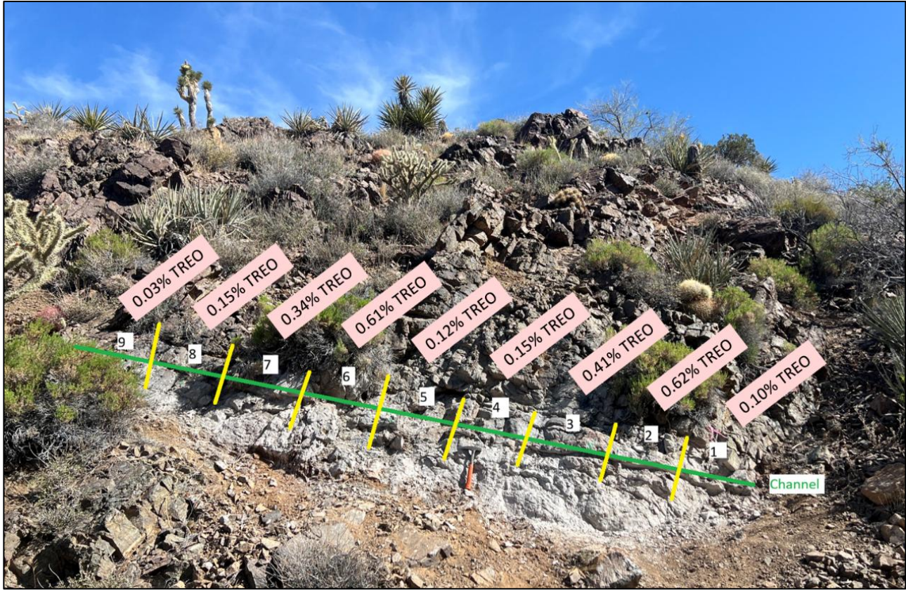
Figure 4: Rock chip channel sample %TREO results from shonkinite outcrop associated with the northern carbonatite (photograph looking north).
