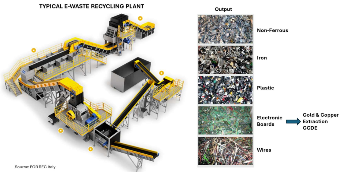
Figure 3 – Typical E-Waste recycling plants separating electronic boards
