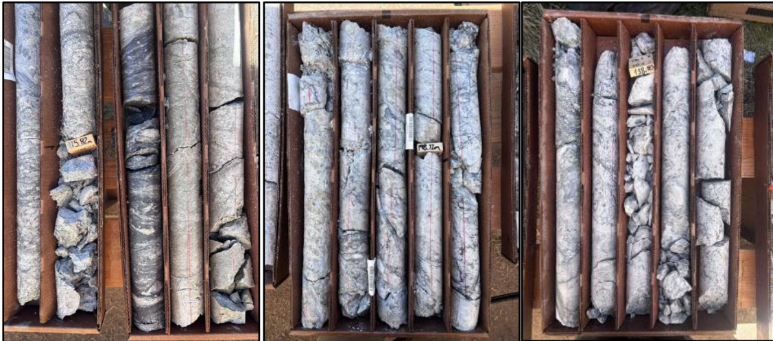
Figure 4: Mineralised and altered drill core in HH-GG26-001C (114-119 ft) & (195-199 ft) and in HH-GG26-002C (137-142 ft) from Golden Gate South (Refer to Appendix A) for sample drill hole locations.
