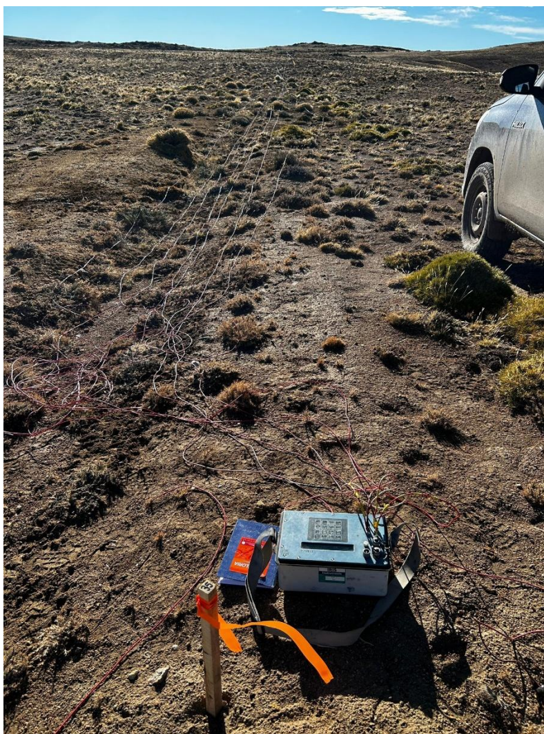
Figure 3 – IP Survey Line Deployment at Sascha Marcelina Project
