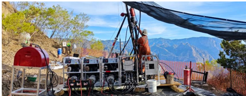
Figure 1. Diamond rig set up at the site of Advance's first drill hole at the Gavilanes Project in Durango, Mexico.
