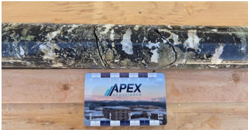
Strong visual zinc-copper sulphide in drill core from WD26-01 (520m)
