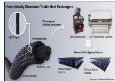
Fig. 3 Hierarchically structured textile heat exchangers — CNTF yarn to woven & knit spacer fabrics.
