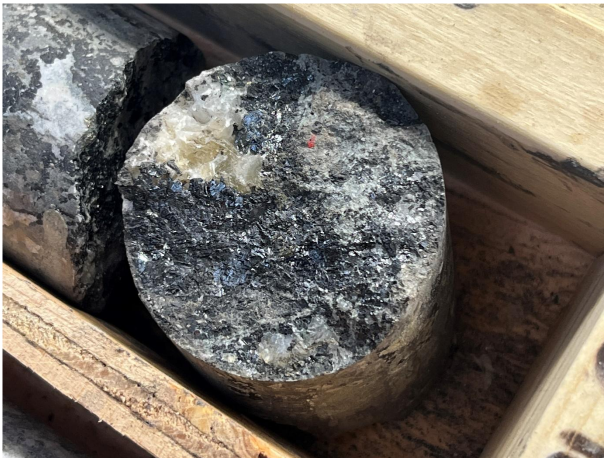
Figure 6: Visual coarse-grained sphalerite (black) within carbonate host rocks in NQ drill core from approximately 505.87m downhole in drill hole WD26-01. Laboratory assays for this interval are pending).
