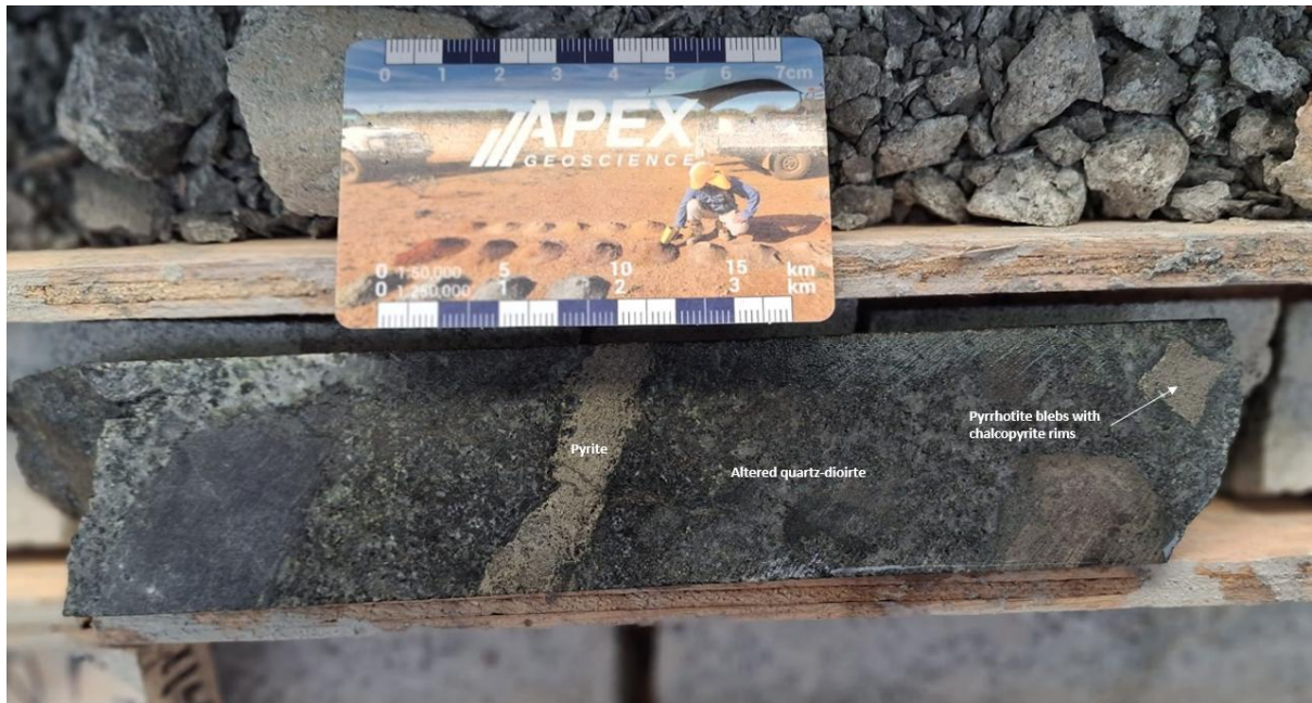
Figure 10: Visual pyrrhotite and chalcopyrite blebs and disseminations within altered quartz-diorite, overprinted by pyrite veining in NQ drill core from approximately 356.95m downhole in drill hole WD26-01. Laboratory assays for this interval are pending.
