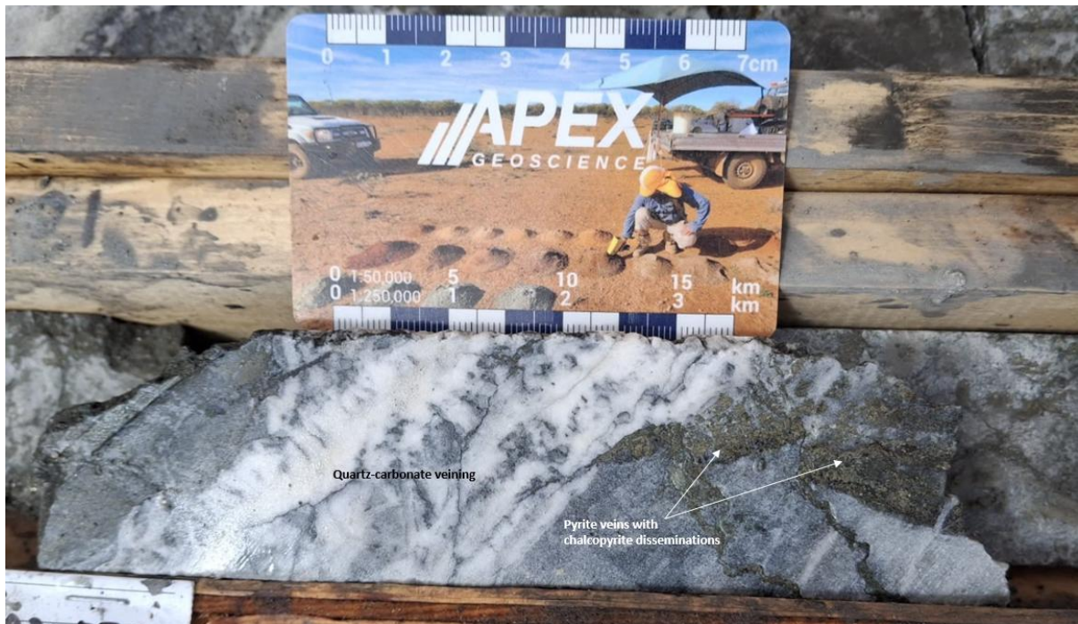
Figure 11: Visual silica-carbonate veining overprinted by pyrrhotite-hematite-chalcopyrite veins, hosted within exoskarn limestone in NQ drill core from approximately 578.95m downhole in drill hole WD26-01. Laboratory assays for this interval are pending.
