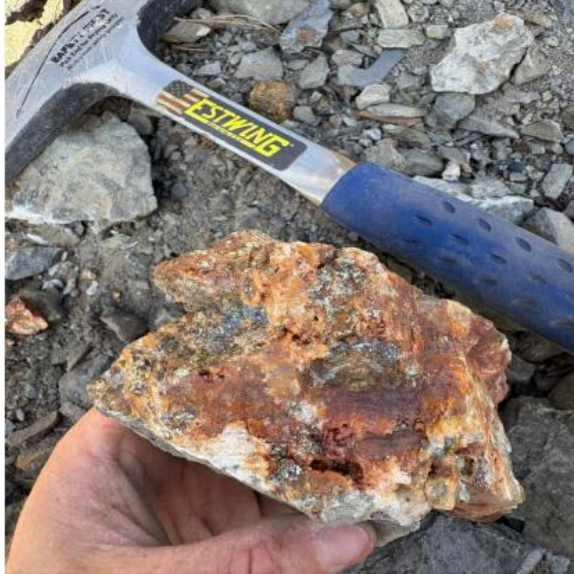
Figure 5. Rock Sample GR019 from Davis Mine prospect - Grading 1.96% Cu, 1.465% Zn 0.29% Pb
