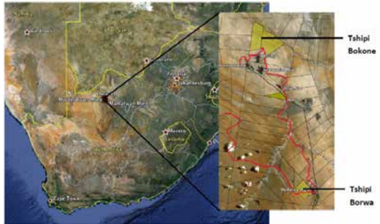
The Tshipi Borwa Mine is located on the south western outer rim of the Kalahari Manganese Field making the ore resources shallower and more amenable to open pit mining.
