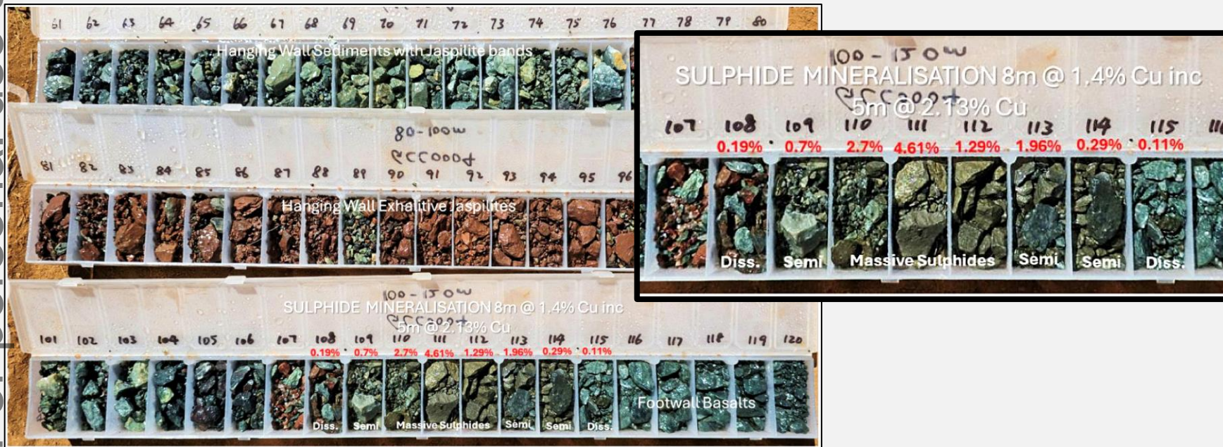
Chip Trays from Hole GC0004 showing the classic VMS stratigraphic succession from hanging wall sediments, jaspilite, disseminate to semi-massive to massive sulphides to footwall basalts.
