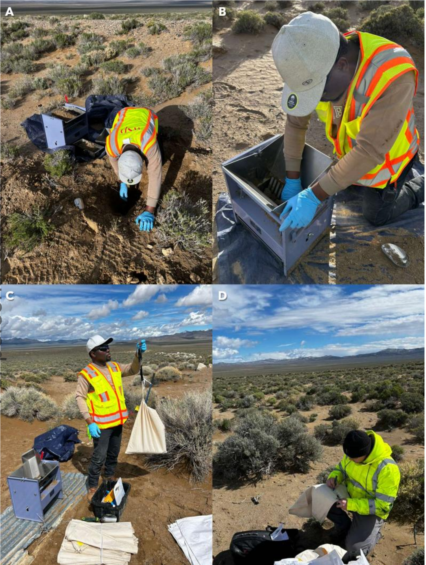
Figure 3; Photos showing; A: Sample collection, B: riffle splitting sample, C: bagging of sample & D: preparing sample bags and data recording.
