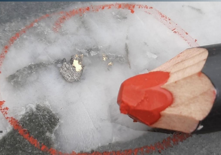
Visible gold from AMD003, which returned 7.5 metres at 55.0g/t Au from 178.1m down hole (ASX AVM 26 September 2025)
