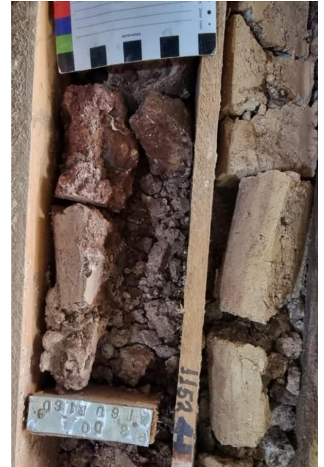
Half drill core from drillhole MFSR-44 with 2m at 85,557ppm (or 8.56%) TREO from 6m.
