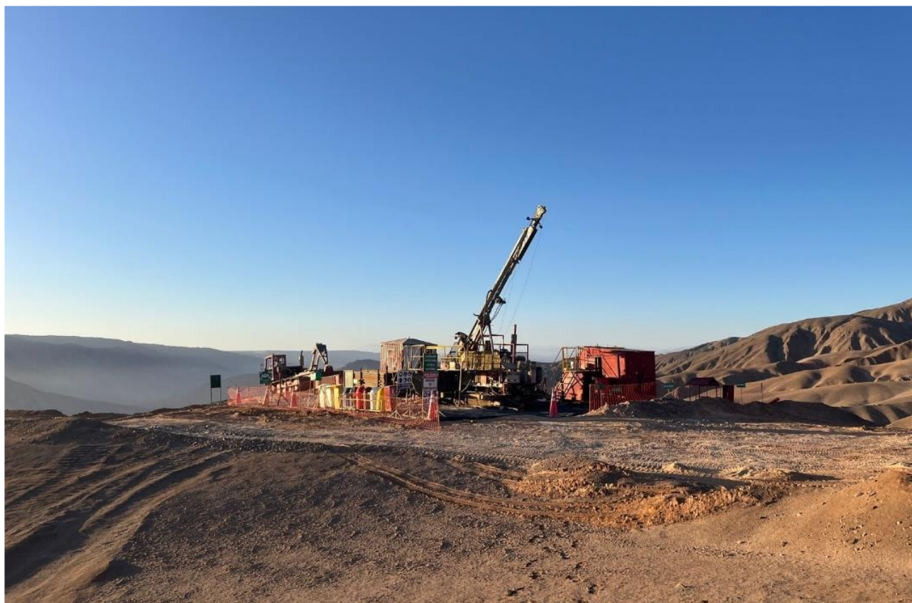
Figure 7: Diamond drill rig operating at Ilo Este, Peru
