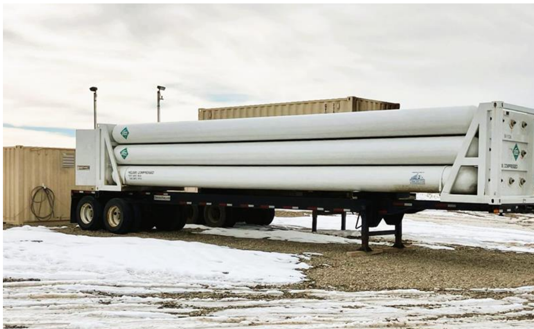
Figure 4: First helium tube trailer on site at the Pinon Canyon Plant
