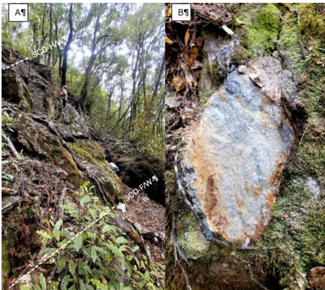
Figure 7: A. Outcrop of the Doyles fold showing the hangingwall (H/W) and footwall (F/W). B. SCD footwall showing highly silicified and altered granite with arsenopyrite veinlets shown by dark grey. Rock chip assays obtained from this area have ranged from 1.0 to 9.6 g/t Au.
