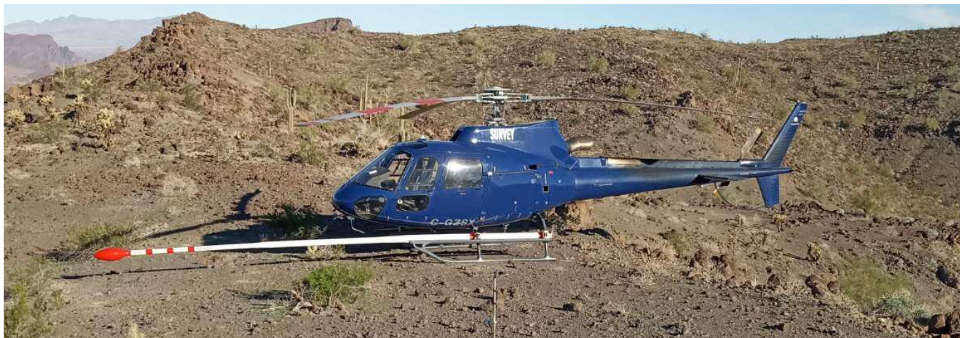
Figure 18 - Helicopter used for the ultra-high resolution airborne aeromagnetic and radiometric survey at the Parker Gold (Cu-Au) Project, shown at the base station magnetometer.
