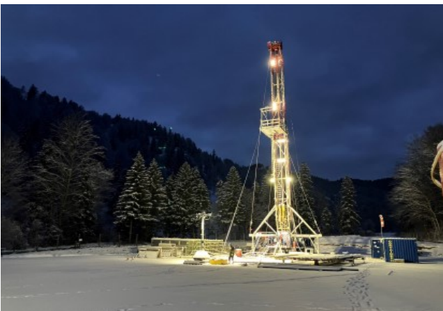
Welchau-1 well testing operations in the ADX-AT-II licence during January 2026 confirming a light oil (46 API) column in the well based on sampling recovered at surface,
