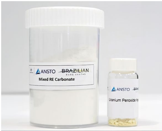
MREC and Uranium Yellowcake Produced by ANSTO from Monte Alto mineralised material.
