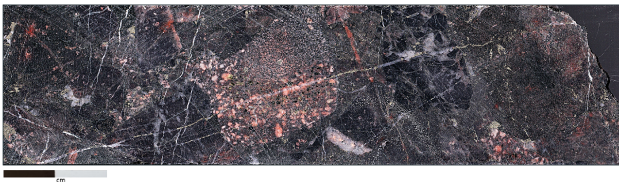
Figure 9: BZD001 - 190 – 191m 6930 ppm Cu, 0.9g/t Au. Magmatic-hydrothermal breccia with strong potassic alteration. Chalcopyrite-pyrite mineralisation hosted within clasts, hydrothermal breccia and porphyry veining
